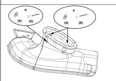
3. Attach the assembled slide runway to the ladder using the hardware shown.
