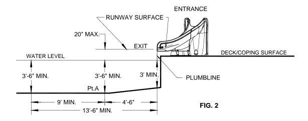
2. A minimum clearance area in front of the slide shall be maintained at all times as follows:
