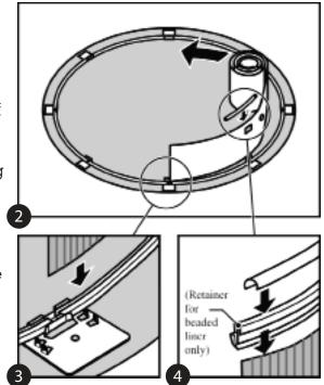
e. Work around the foundation until the entire pool wall is uncoiled into the bottom rails and the top edge is covered with the omega stabilizer and connectors (and beaded liner retainers if you have a beaded pool liner).
