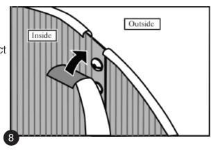
Hint: Stick a screwdriver through two of the holes to help line up the ends of the wall. 3. Make sure the Pool Wall is
