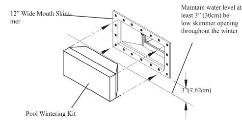
Insert the Pool Winterizing Kit (Part Number 1370138) into the skimmer until it fits flush with the skimmer flange. On some skimmers, it may be necessary to trim the foam to make a friction fit and/or use a wooden wedge to keep it in place during the winter.
