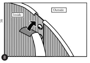
Hint: Stick a screwdriver through two of the holes to help line up the ends of the wall.
