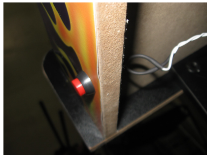
Mounted reset button with approx. 10' wire to attach to scoring harness.
