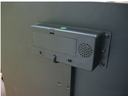
Electronic Scorer mounted on Backboard with digital readout in front. Uses 4 AA batteries.
