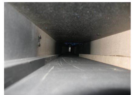
Ball return liners should be firmly glued in place with NO bubbles or wrinkles.
