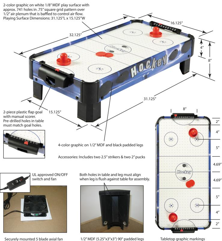
AC120V 50/60 Hz 0.28A 24W 2P w/ a min. 6.5" square mounting board. 1/2" MDF (5.25"x3"x3") 90° padded legs should flush mount to table securely with 2 bolts, washers and nuts. Tabletop graphic markings measurements
