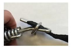
**STEP 1:** Pass the strap under the front of the spring and through the middle of the d-ring.
