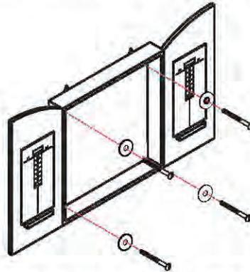
Step 2: Once you are certain the marks are at the proper height and they are located at the wood studs, have someone hold the Dartboard Cabinet (without the **Bristle Dartboard (#1)**) against the wall. Make sure that the four holes in the Cabinet are lined up with your previous pencil marks. Now use an electric screwdriver to screw the **2" Screws (#3)** with **Washers (#4)** directly into the wall making sure to drill into the wood studs.
