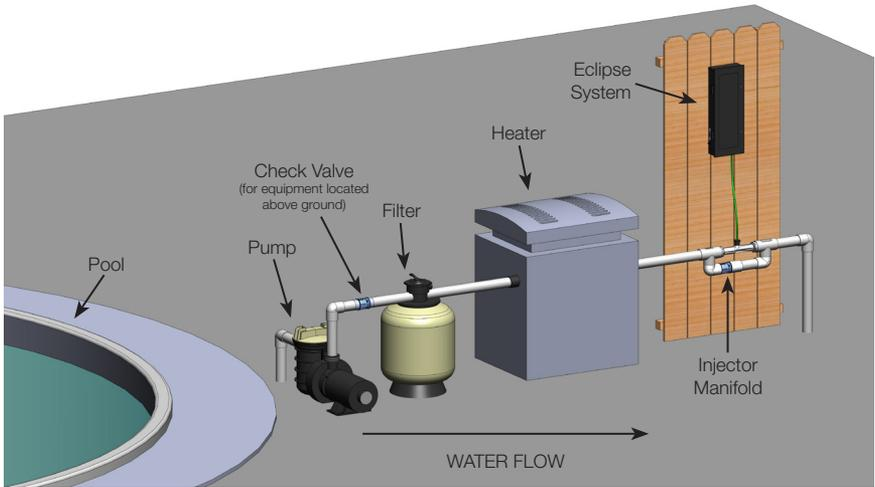
**Figure 2: Injector Manifold Mounting Location**
