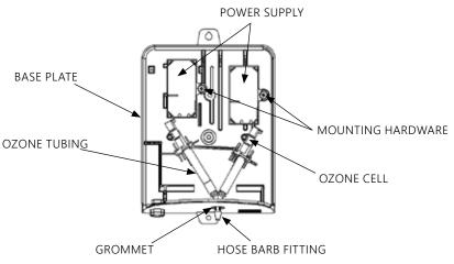
Figure 6: Internal Component Locations
