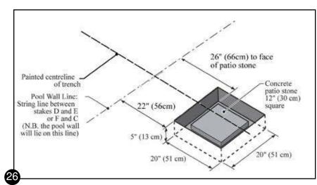
k. Temporarily replace the strings removed in step (i) to check that the trenches are exactly parallel. Remove the strings again when you are finished.
