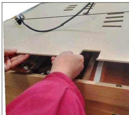
FIG 17 Slip the power cord through Roof Cover
