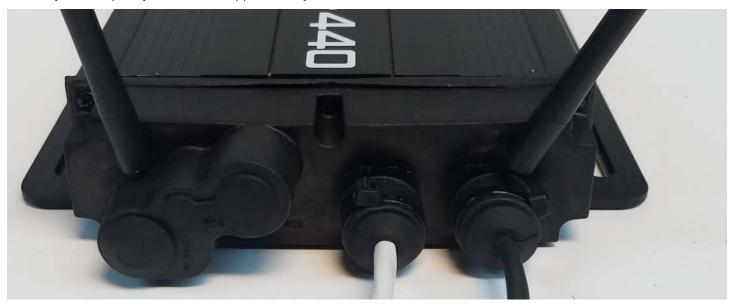
NOTE: Optical and RCA inputs are not intended to be used in a permanent outdoor setting. Both optical and RCA inputs require a separate media source, which is more than likely not resistant to weather.
