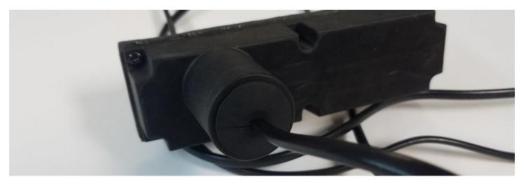
4. Use one of the supplied nylon zip ties and tighten the zip tie around the plugged opening. Tighten the zip tie to the point where the inside of the rubber body begins to deform and looks similar to the image below. Hold up to light to verify a good seal was formed.
