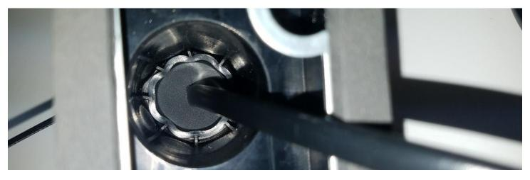
5. Plug the power cord into the OS-440, adjust the power cord length as needed. Secure the rubber body to the OS-440 by lining up the gasket over the outside edge of the OS-440 chassis and use the four (4) of the 7/16" long machine screws and evenly tighten each screw with a Philip's head screwdriver to create a good seal. Retighten the zip tie until it indents the rubber.
