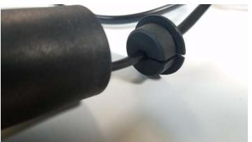
3. Now massage the rubber plug around the power cord into the opening in the rubber body. Use the OS-440 and approximately gauge the length of cord that is through to plug.
