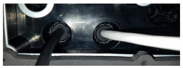
6. Carefully adjust the slack in each of the speaker cables so that they run straight out the ports. Speaker cables are not to be coiled up within the rubber body. Secure the rubber body to the OS-440 by lining up the gasket over the outside edge of the OS-440 chassis and use the four (4) provided ~1/2 inch machine screws and evenly tighten each screw with a Philip's head screwdriver to create a good seal. Retighten the zip ties as needed until they indent the rubber.
