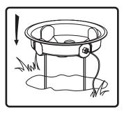
4. Place speaker base into hole in ground with the top rim of the base at ground level. Backfill dirt into hole, packing firmly. For added security, cement security brackets into ground.
