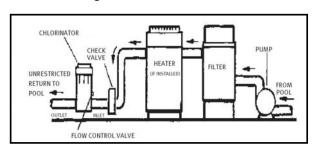
**A CAUTION** Damage to the heater or filter may result if concentrated chlorine is allowed to flow through them.
