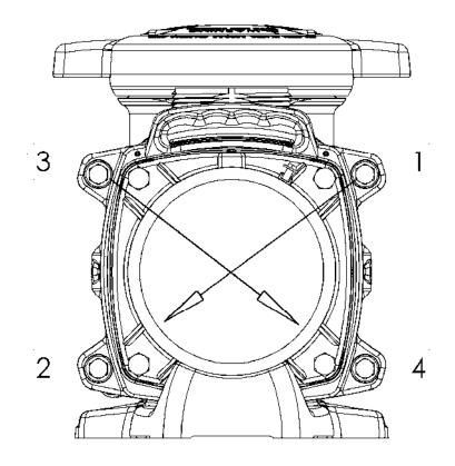
HOUSING BOLT TORQUE PATTERN Fig 7.6.1
