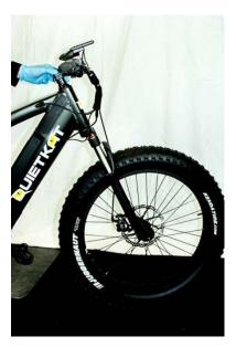
d. Using your 5mm Allen key or Torque Wrench, tighten all stem bolts to 7nm (Newton Meters).
