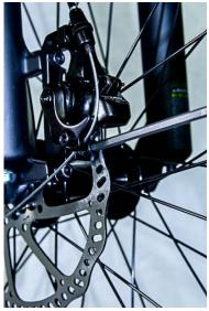
f. With the Brake Caliper slightly loose, squeeze the front brake lever to engage the pistons and squeeze the rotor with the pads; keep it squeezed while tightening the Brake Caliper bolts. Release the brake lever and spin the wheel to ensure the rotor is centered within the pads. You can make fine adjustments to the inside pad position with a 5mm Allen key on the side of the brake caliper.
