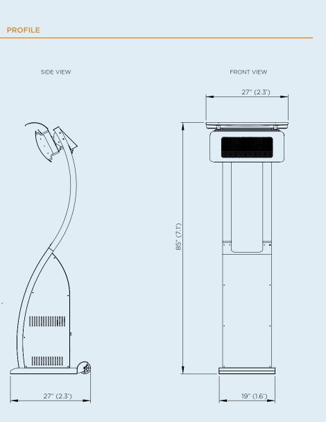
Measurements displayed within this document are minimum requirements for installation. Bromic takes no responsibility for incorrect or non-compliant installations. All measurement in this document are displayed in inches.
