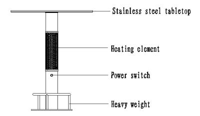
Use power switch to control heating element on/off
