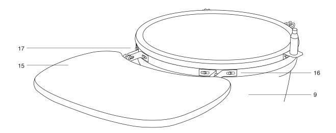
**STEP 16 -** Insert the 2x table hinge into each of the table brackets (16 & 17).
