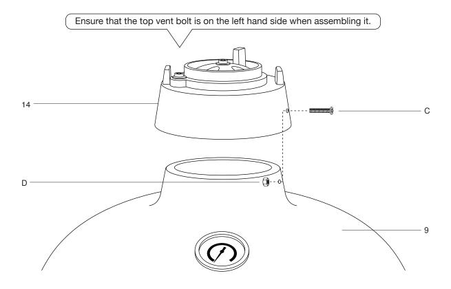
STEP 13 - To attach the top vent (14) to the Kamado Grill (9) place it on top and align both the bolt holes. Secure using 2x bolts (C) and nuts (D) Ensure that the top vent bolt is on the left hand side when assembling it.
