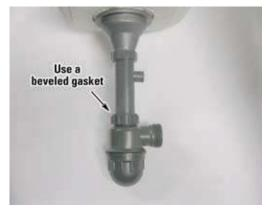
8. Attach drain elbow (7).
