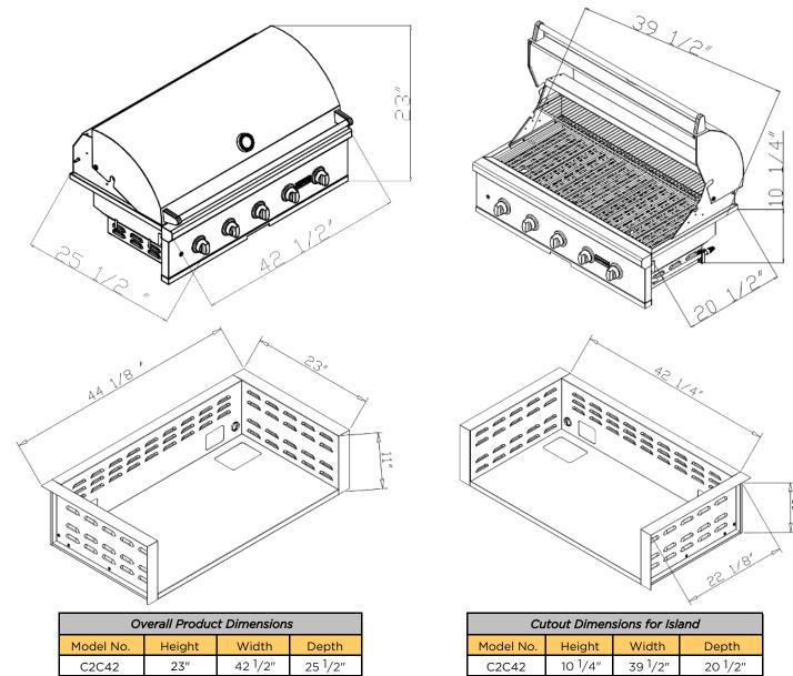
✓ When using a Coyote insulated jacket, you will want to build your island to the jackets Cutout and Overall Dimensions listed above. Once the jacket is installed, the grill will rest on/inside the insulated jacket
