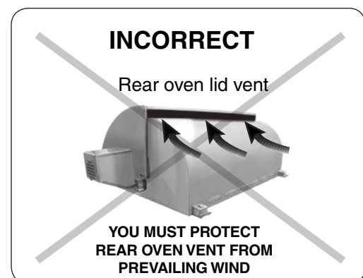
Fig. 10-3 Airflow direction - INCORRECT
