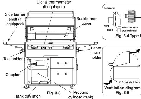
Fig. 3-4 Type I Acme thread coupler To connect the regulator/ hose assembly to the propane-gas cylinder valve fitting: Press the hand nut on the regulator over the Acme thread fitting on the cylinder valve. Turn the hand nut clockwise to
