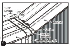
along to shorten the transition rail. The seconde line  $\mathbf{Y}$  is also parallel to the end of the side rail, 1-1/8" (29mm) away. this will be the line that the new 1/4" (6mm) screw holes lie on.
