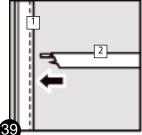
tabs at the end **W** of the diagonal into the slots in the upright (key 1) (see diagram 39).
