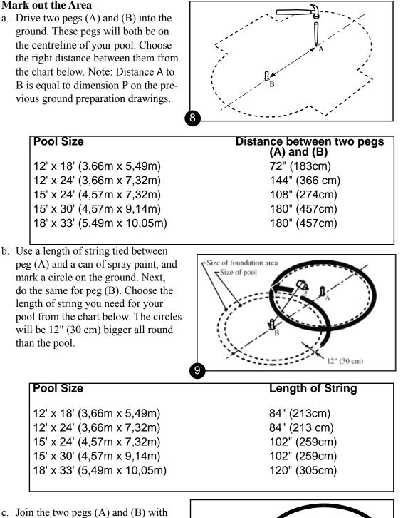
c. Join the two pegs (A) and (B) with a piece of string. Use this string as a guide to paint your centreline on the ground with the can of spray paint.
