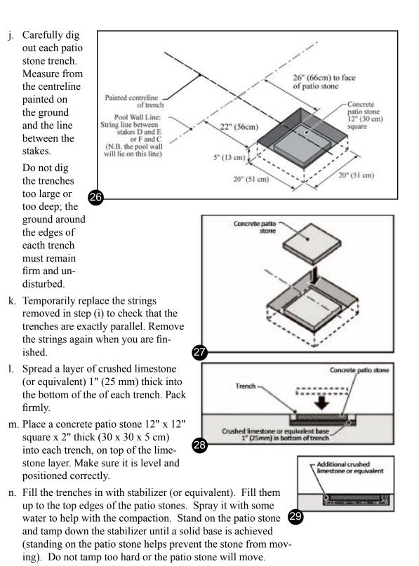
o. Recheck the distances between the patio stone and make any adjustments you need to make sure the spacing is exactly right. Refer to page 1-10, Step 6 for measurements.
